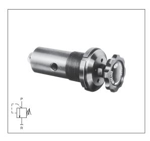
The pilot-operated relief valve is mainly used for remote control of the main circuit pressure by connecting it to the vent port (VE) of a balance piston type relief valve. In a small-flow circuit, this type of valve can also be used as a direct acting type relief valve.
